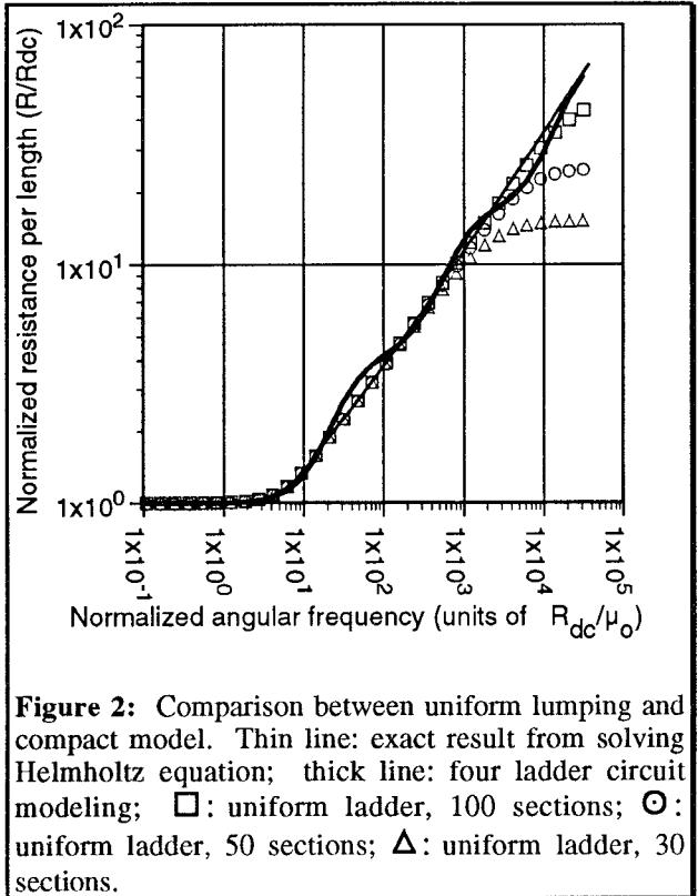
**Figure 2:** Comparison between uniform lumping and compact model. Thin line: exact result from solving Helmholtz equation; thick line: four ladder circuit modeling;  $\square$ : uniform ladder, 100 sections;  $\circ$ : uniform ladder, 50 sections;  $\Delta$ : uniform ladder, 30 sections.
