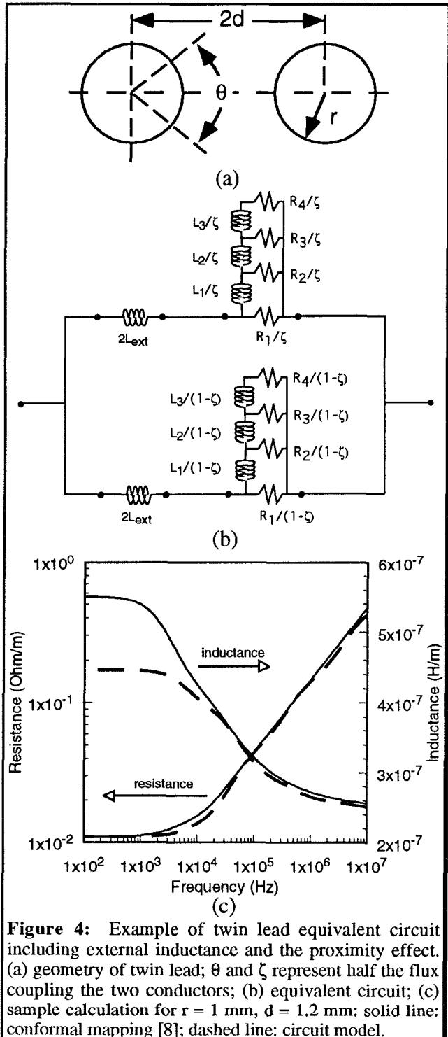
**Figure 4:** Example of twin lead equivalent circuit including external inductance and the proximity effect. (a) geometry of twin lead;  $\theta$  and  $\zeta$  represent half the flux coupling the two conductors; (b) equivalent circuit; (c) sample calculation for  $r = 1$  mm,  $d = 1.2$  mm; solid line: conformal mapping [8]; dashed line: circuit model.
