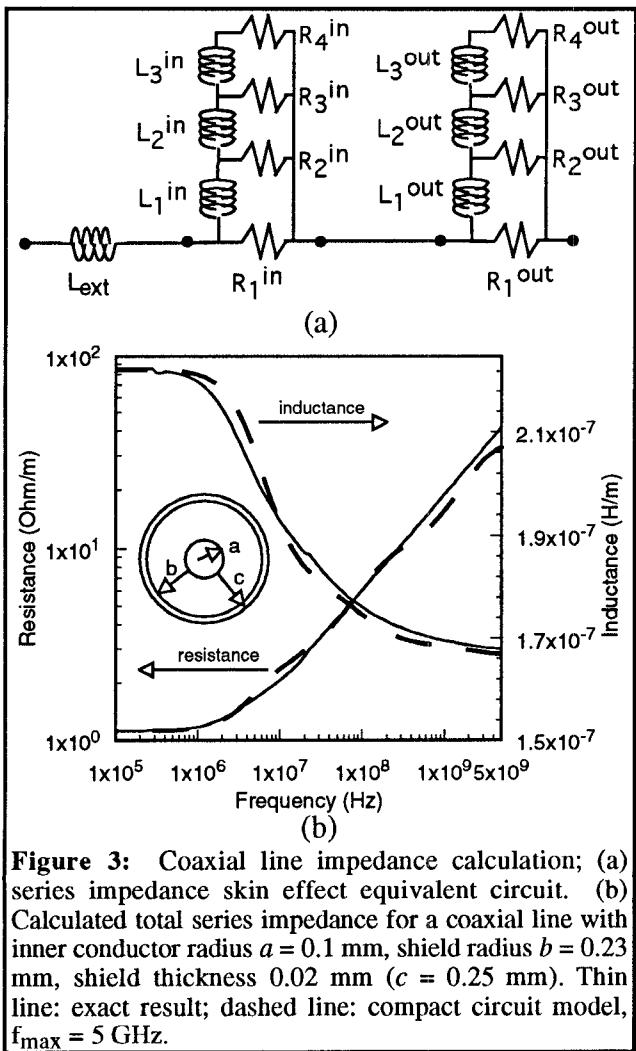
Figure 3: Coaxial line impedance calculation; (a) series impedance skin effect equivalent circuit. (b) Calculated total series impedance for a coaxial line with inner conductor radius  $a = 0.1$  mm, shield radius  $b = 0.23$  mm, shield thickness 0.02 mm ( $c = 0.25$  mm). Thin line: exact result; dashed line: compact circuit model,  $f_{max} = 5$  GHz.
