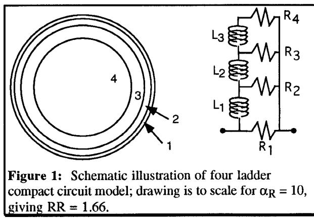
Figure 1: Schematic illustration of four ladder compact circuit model; drawing is to scale for  $\alpha_R = 10$ , giving  $RR = 1.66$ .
